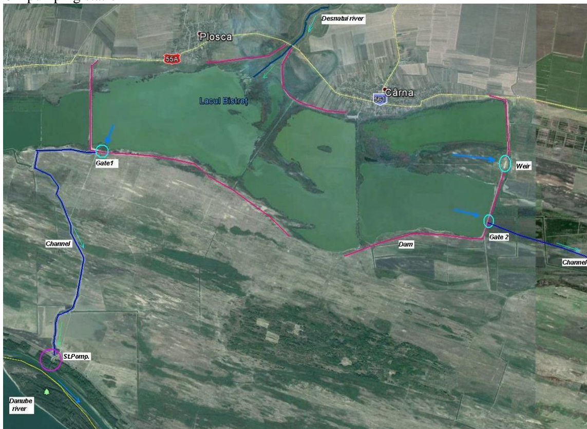
Figure 10. Plan of the location and of the major hydrotechnical works of Bistret Lake.
